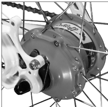
Rohloff SPEEDHUB 500/14 CC OEM2 mounted with the support bolt
