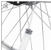
Remove the drain screw (3mm allen key) and fit the filling tube and syringe. Turn the wheel, so that the filling point is underneath the hub. Wait approx. 15mins with the wheel in this position, then draw out the old fluid. Remove the syringe and filling tube and pour the fluid into the 50ml cleaning oil bottle.
