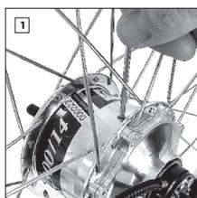
To change the oil, the hub should be left at room temperature (because the oil flows better). Turn the hub, so that the drain screw can be seen on the top. Remove drain screw (3mm allen key).
