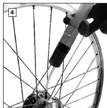
Draw 25 ml SPEEDHUB OIL into the syringe and insert it into the hub. Draw out approx. 15ml of air to keep the pressure correct inside and therefore, avoid oil seeping back out, when removing the filling tube.
